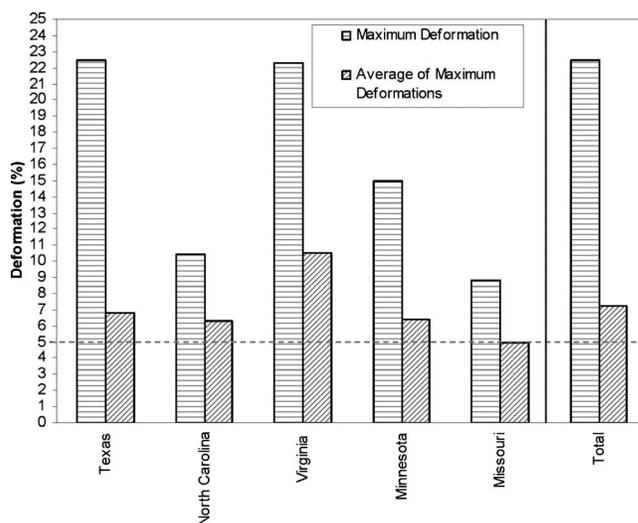
**Fig. 7.** Maximum and average values for maximum deformations of pipelines inspected in each state and the average and maximum of the total pipes inspected
