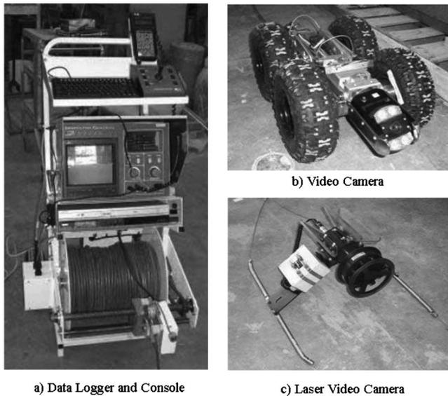
**Fig. 1.** Different instruments used in pipeline inspections: (a) CUES inspector general instrumentation console; (b) CUES rover with OZII pan/tilt/zoom camera module (P/N CZ902); and (c) 10-head laser ring and skid
