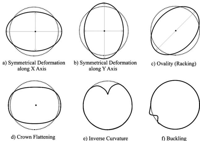
**Fig. 4.** Different types of observed deformation types (schematic view)
