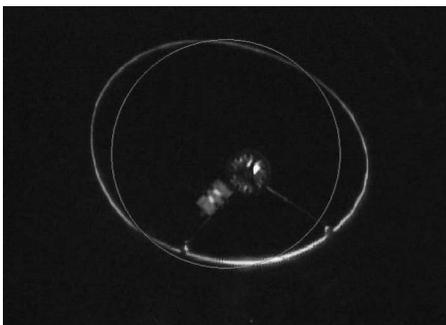
**Fig. 2.** Example view of laser ring on deformed surface of a pipeline compared to the original undeformed shape of the pipeline section
