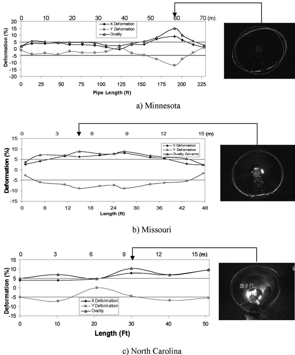
**Fig. 10.** Vertical, horizontal, and ovality deformations along the length of pipelines in different states and corresponding views of sections showing the laser ring profile on the deformed shape of the section compared with the original undeformed ring
