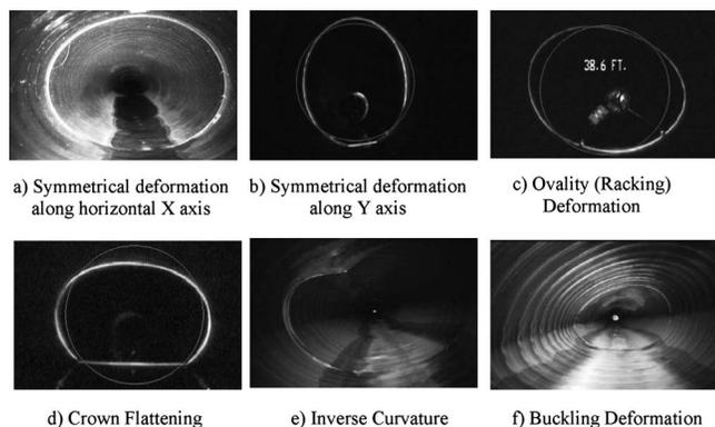
**Fig. 5.** Different types of observed deformation types (real examples)
