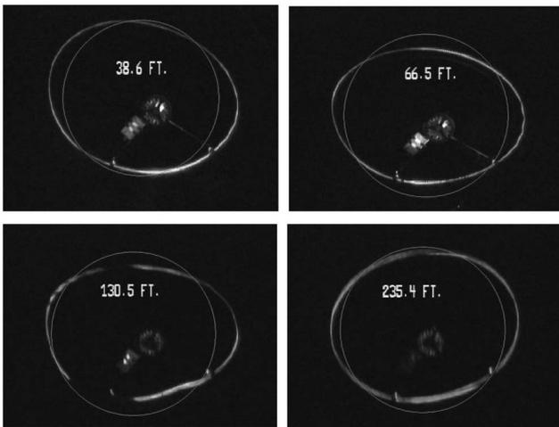
**Fig. 8.** Vertical, horizontal, and ovality deformations along the length of a pipeline and corresponding views of sections showing the laser ring on deformed shape of the section compared with the original undeformed ring for a 36 in. (91.44 cm) pipeline
