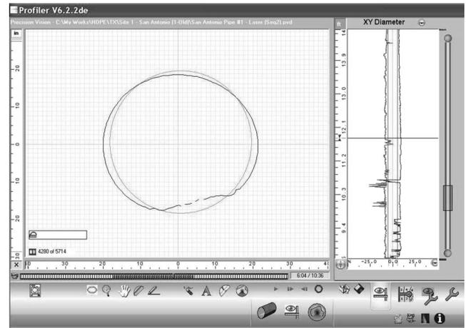
**Fig. 3.** View of the Profiler software used for analyzing the pipeline deformation graphs showing the original undeformed shape of the pipeline section surface and the captured deformed shape of the section on the left side of the figure and deformation graph on the right side of the figure
