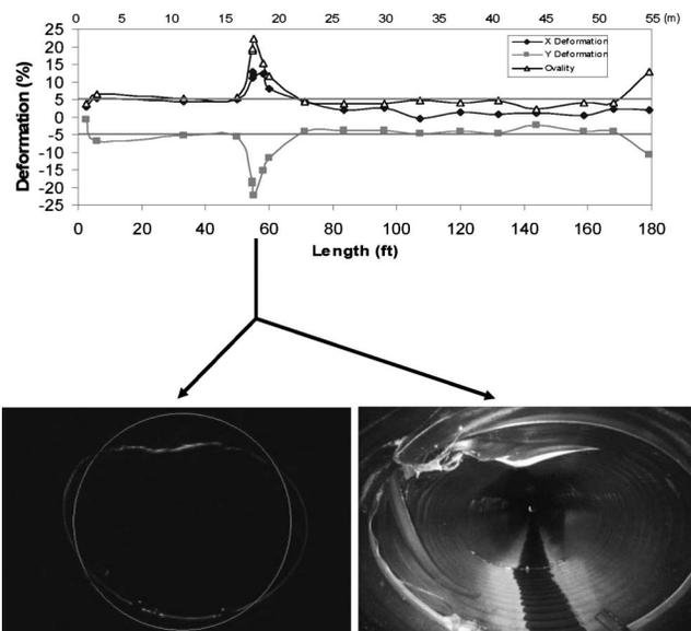
**Fig. 9.** Vertical, horizontal, and ovality deformations along the length of a 36 in. (91.44 cm) pipeline showing the laser ring on deformed shape of the section compared with the original undeformed ring and snapshot of the section showing the maximum deformation along the length of the pipeline
