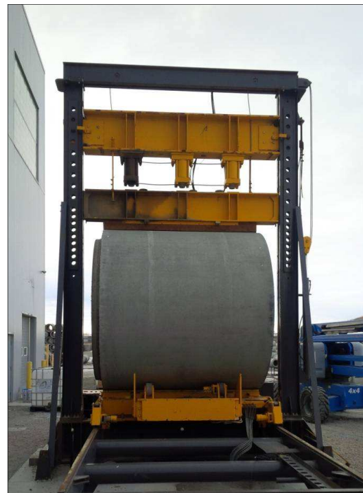
Figure 3: Three Edge Bearing Tester used to confirm pipe strength
