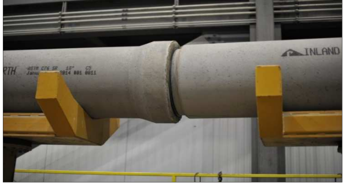
Figure 4: RCP undergoing a Hydrostatic Test
