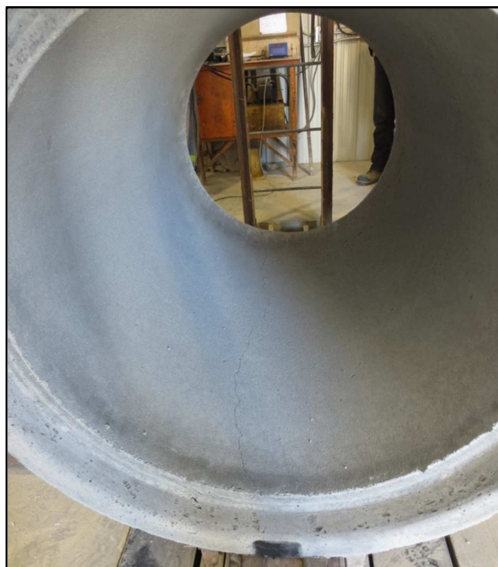
Figure 3 (left): Flexural Failure in Three-Edge Bearing Machine Test
